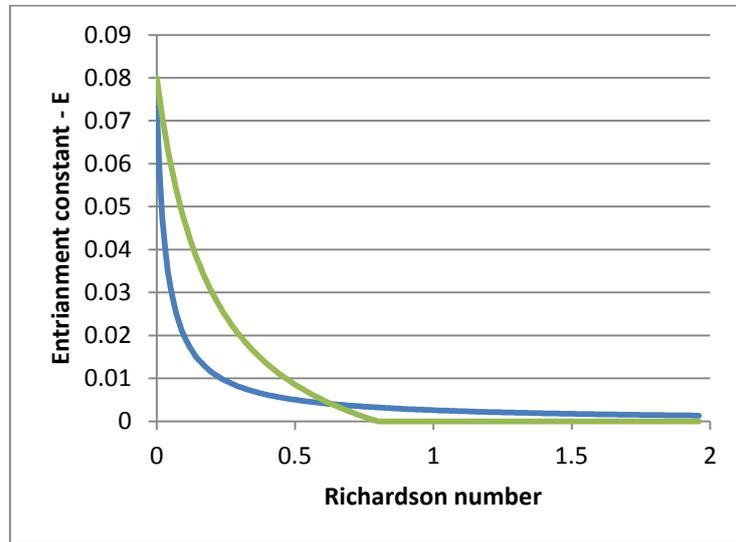
Figure 4: Entrainment constant as a function of Ri
