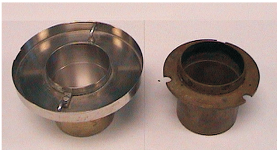
Figure 4. Flash point apparatus modified cup (left) and standard cup (right)
