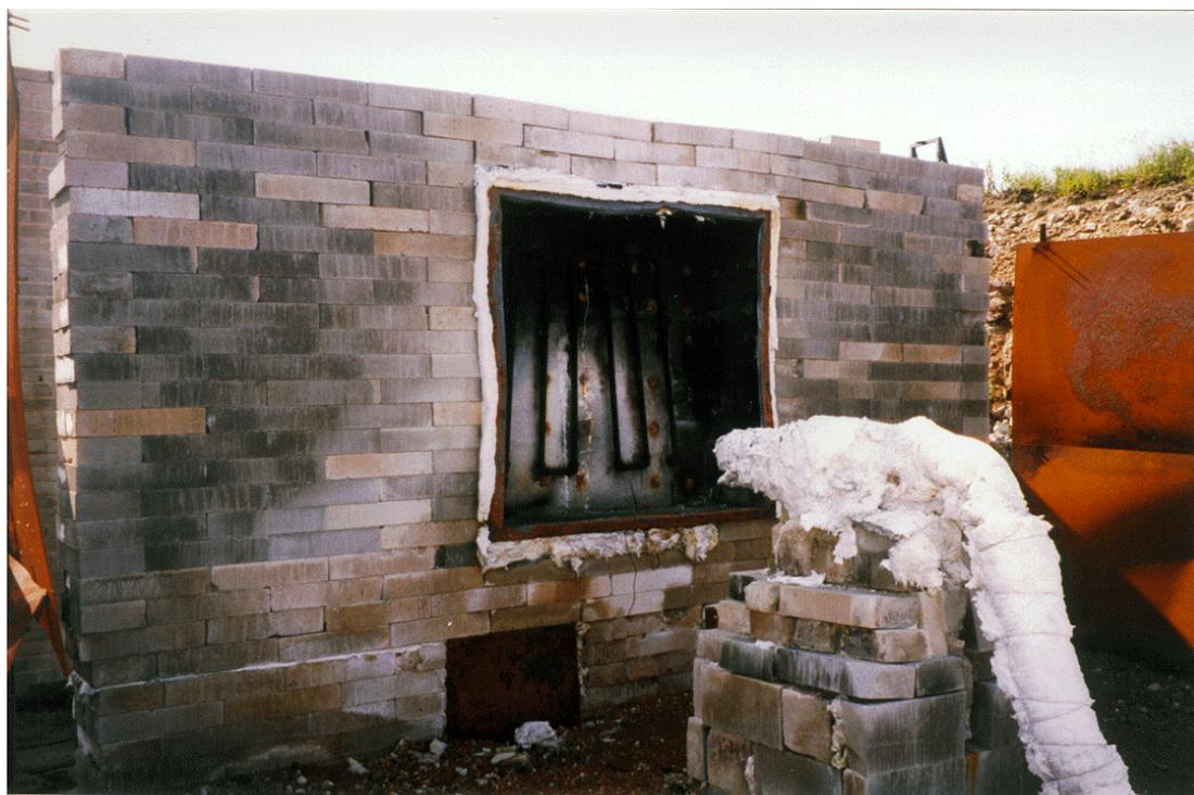
**Figure 4. PIPE CALORIMETER IN POSITION**
