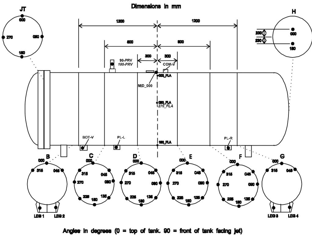
Figure 7. THERMOCOUPLE POSITIONS ON PROPANE TANK
