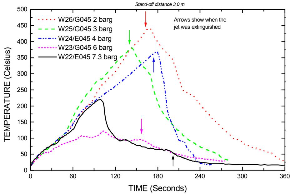
**Figure 8. MAXIMUM SHELL TEMPERATURES VS. WATER DELUGE PRESSURE (Recommended minimum rate system with 3.0 m propane stand-off)**
