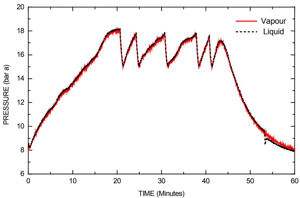
**Figure 11. PROPANE VAPOUR AND LIQUID PRESSURES**
