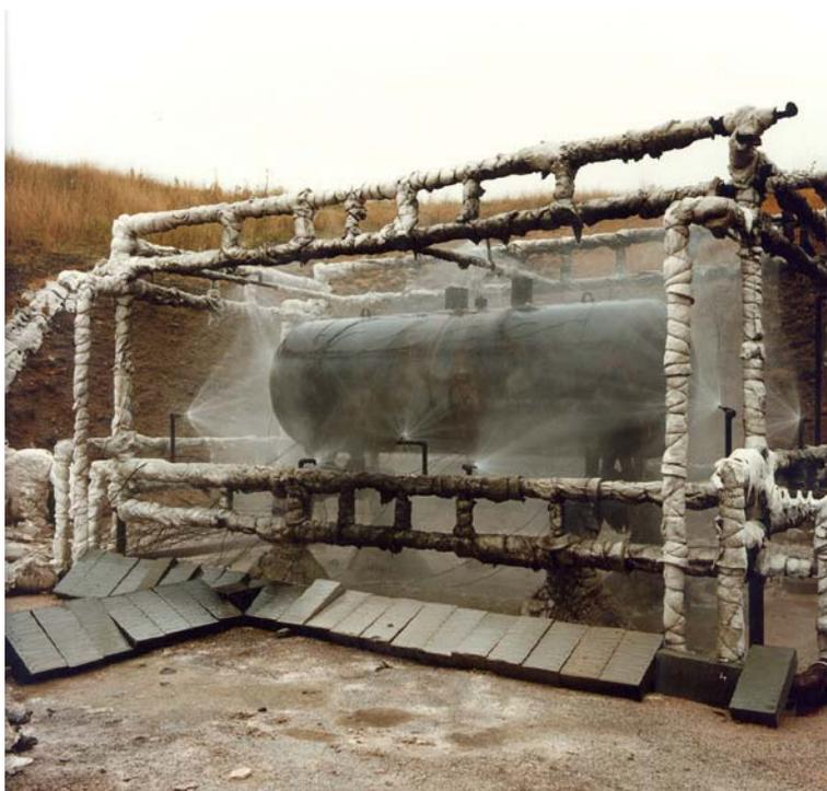
**Figure 4. MINIMUM RATE SPRAY PATTERN ON UNPRESSURISED VESSEL**
