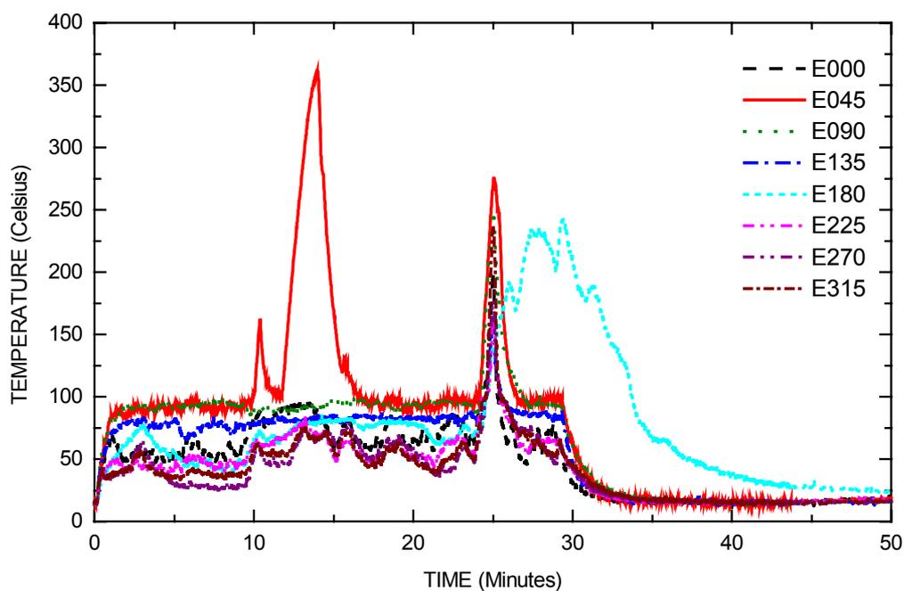
**Figure 12. EMPTY TANK BAND E SHELL TEMPERATURES (Tentative Rule system with 3.0 m propane stand-off)**
