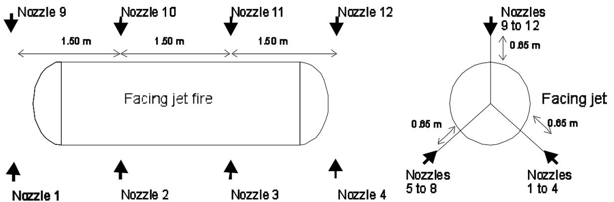
**Figure 3. NOZZLE ARRANGEMENT TO GIVE TENTATIVE RULE RATE**
