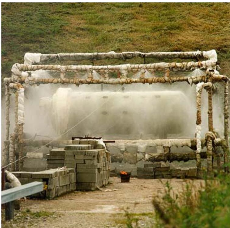
**Figure 5. TENTATIVE RULE SPRAY PATTERN ON 20% FULL PROPANE TANK**
