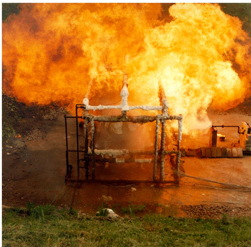
**Figure 10. FIRE ENGULFMENT OF 20% FULL PROPANE TANK**
