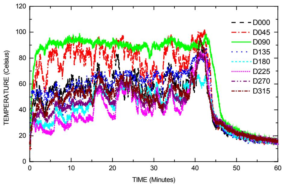
**Figure 9. 20% FULL PROPANE TANK: MAX. BAND D SHELL TEMPERATURES (Tentative Rule system with 3.0 m propane stand-off)**
