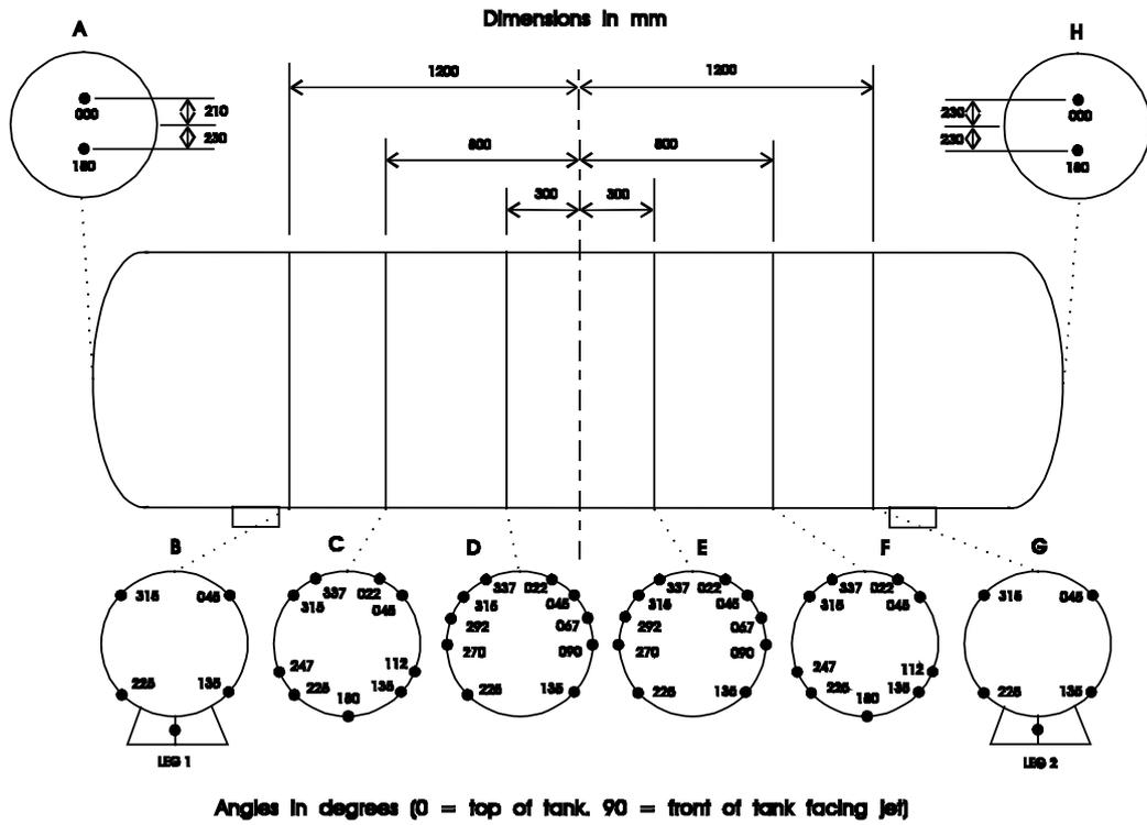
Figure 6. THERMOCOUPLE POSITIONS ON UNPRESSURISED VESSEL
