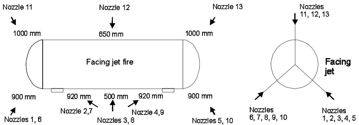
**Figure 2. NOZZLE ARRANGEMENT TO GIVE HSE MINIMUM RATE**
