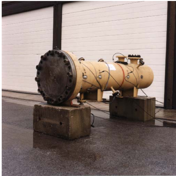
Figure 1 The instrumented heat exchanger before installation in bunker
