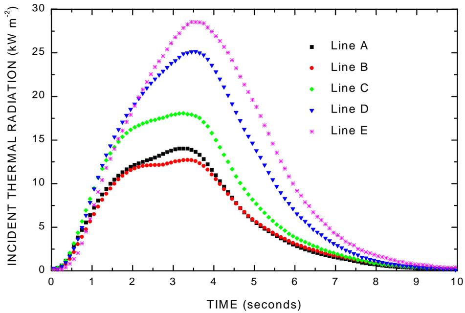
**Figure 4. VARIATION OF IRRADIANCE AT 100 METRES (FOR 1708 KG RELEASE)**
