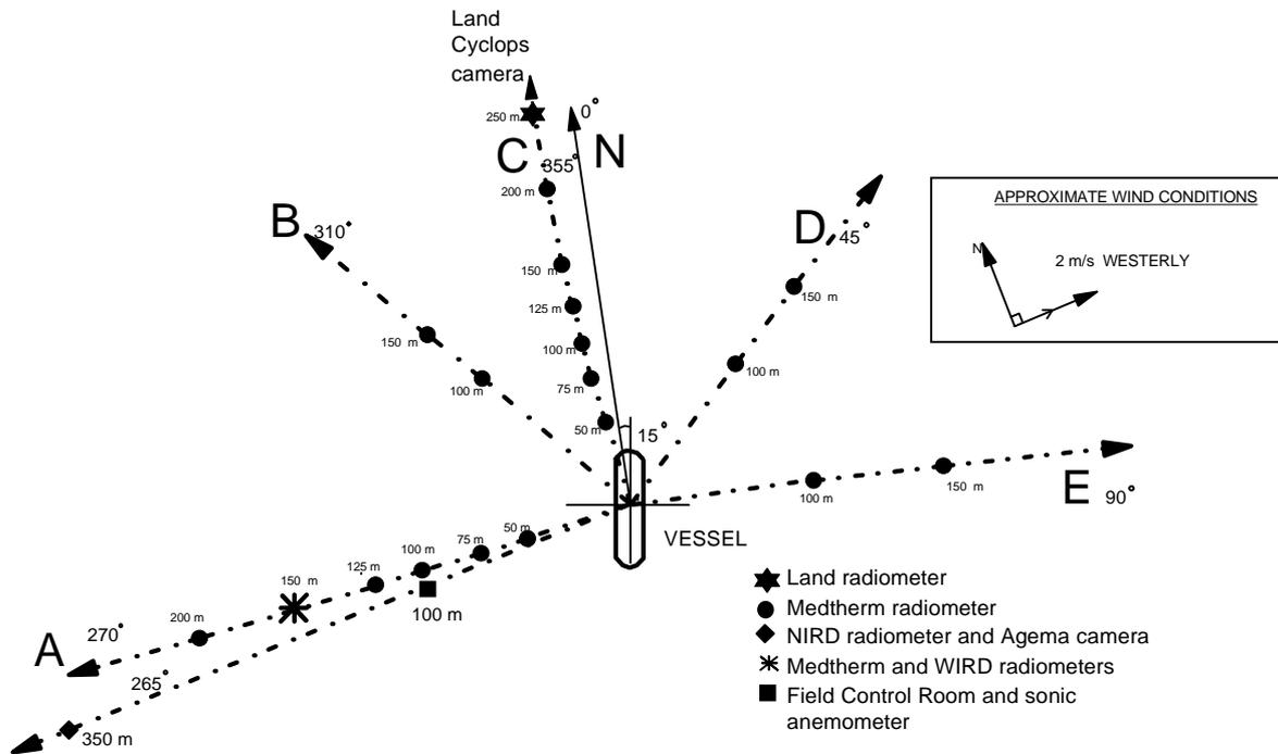
**Figure 1. INSTRUMENT PLAN FOR 1708 KG RELEASE**
