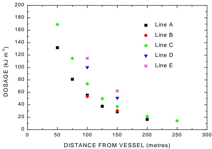
**Figure 5. VARIATION OF DOSAGE AGAINST DISTANCE (FOR 1708 KG RELEASE)**
