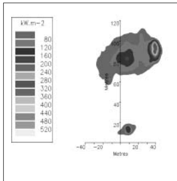
**Figure 3. THERMAL IMAGES FOR 1708 KG FIREBALL GROWTH**
