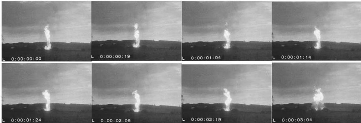
Figure 4. Selected video frame sequences; 85% fill PRV and crack discharge flares, time in seconds to commencement of BLEVE.
