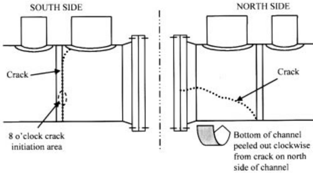
Figure 3 Schematic Representation of the Failure<sup>1</sup>
