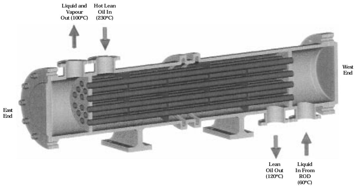
Figure 2 Schematic View of GP905<sup>1</sup>
