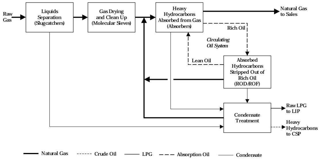
Figure 1 Simplified Overview of GP1 Process<sup>1</sup>
