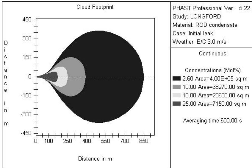
Figure 5 Footprint of Base Case Fully-Developed Cloud
