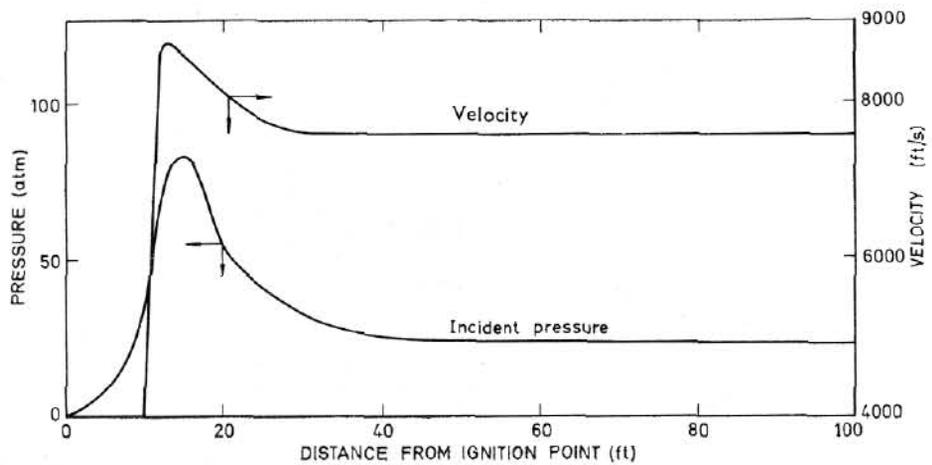
Fig. 5.—Comparison of hydrostatic pressure (pressure gauge at right angles to direction of propagation) measured with pitzo-electro gauge at various distances in 50:50 ammonia-nitrous oxide mixtures
