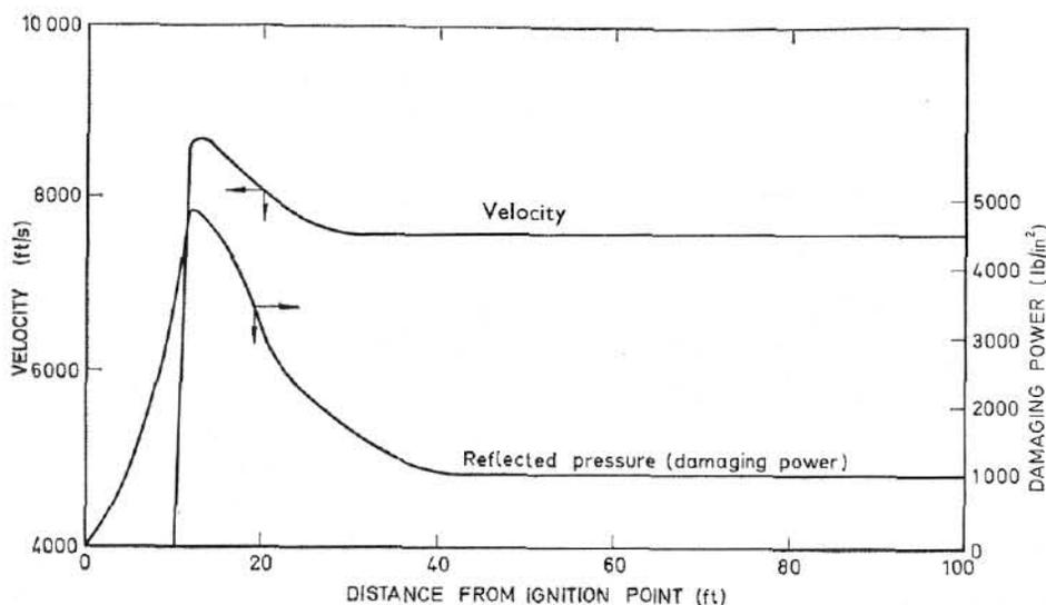
Fig. 6.—Comparison of velocity and damaging power of explosions in 50:50 ammonia/nitrous oxide mixtures in a 3 in. nominal bore pipe
