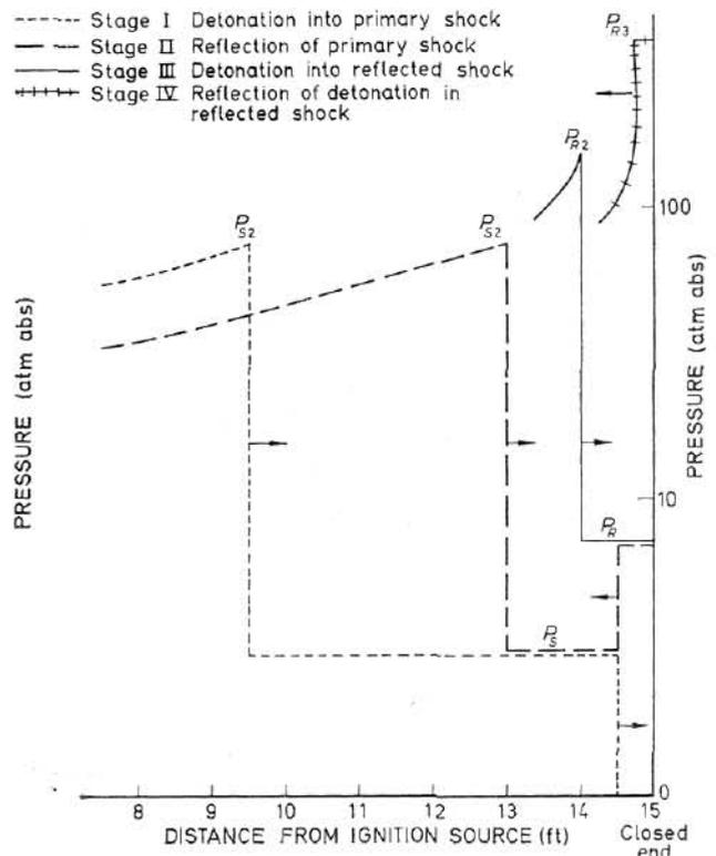
Fig. 12.—Diagrammatic representation of the final stages of the approach and reflection of the overdriven detonation
