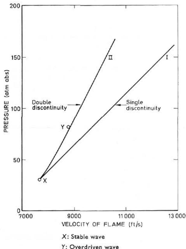
Fig. 10.—Comparison of pressure and velocity of flame propagation of single and double discontinuities
