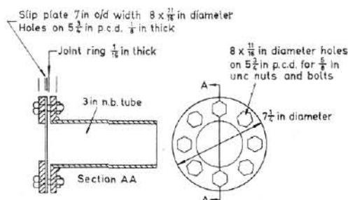
Fig. 2.—Arrangement for holding test plates
