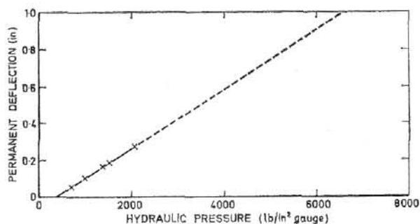
Fig. 3.—Hydraulic pressure calibration of test plates used for measurement of damaging power
