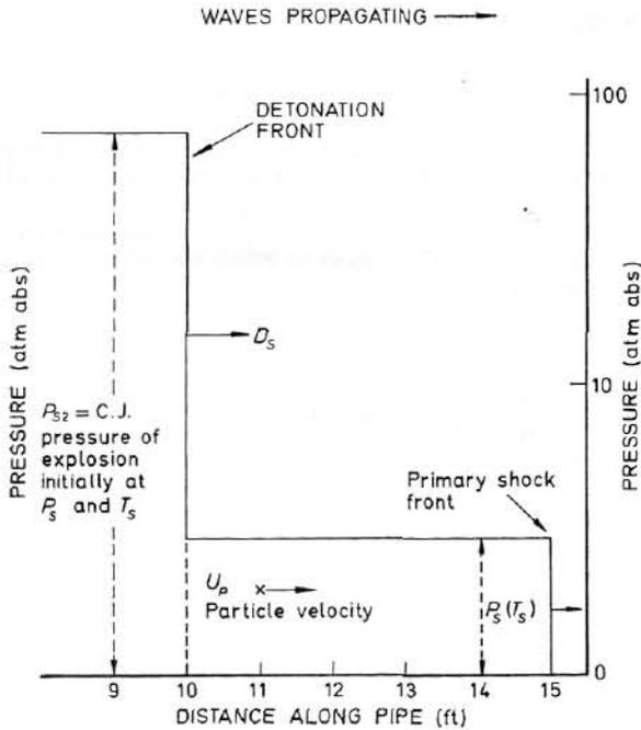
Fig. 11.—Simplified model of overdriven detonation wave: double discontinuity. After Turin and Huebler
