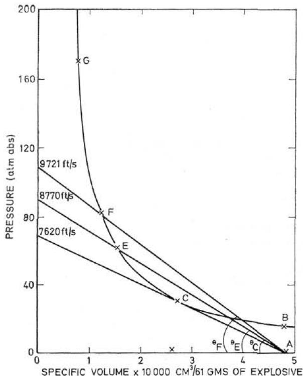
Fig. 9.—Rankine-Hugoniot curve for reactive shock waves in 50:50 ammonia-nitrous oxide mixtures initially at 1 atm pressure and 18°C
