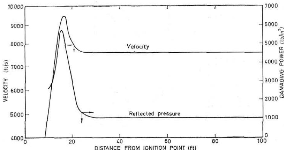
Fig. 8.—Comparison of velocity and damaging power of explosions in 50:50 ammonia-nitrous oxide mixtures in a 4 in. nominal bore pipe
