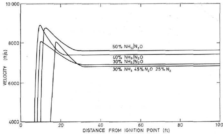
Fig. 4.—Change of velocity with distance travelled by explosions in various mixtures of ammonia-nitrous oxide and nitrogen in 3 in. nominal bore pipe
