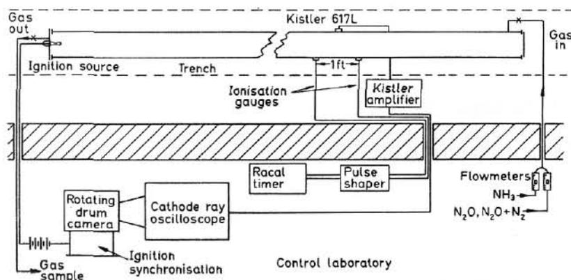
Fig. 1.—Layout of the detonation tube
