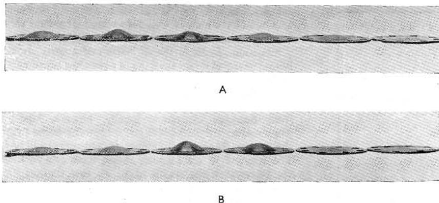
Fig. 7.—Permanent distortion of  $\frac{1}{8}$  in thick test plates resulting from detonations of 50:50 ammonia-nitrous oxide mixtures in various lengths of 3 in. and 4 in. nominal bore pipe
