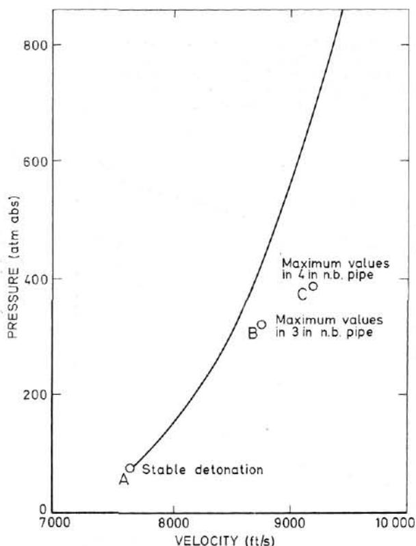
Fig. 13.—Comparison of velocity of flame propagation and pressure developed on reflection of double discontinuity
