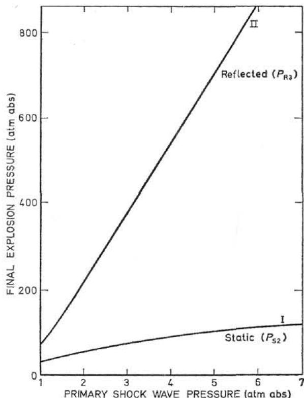
Fig. 14.—Theoretical final pressures (static and reflected) of 50:50 ammonia-nitrous oxide explosion compared with primary shock pressure in the double discontinuity
