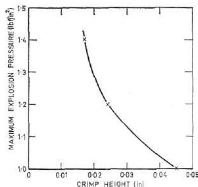
Fig. 8.—Variation of maximum explosion pressure with crimp height for  $1 \text{ ft}^3$  vessel fitted with four vents ( $K = 9.0$ ) and cupro-nickel arresters of  $2\frac{1}{4}$  in. diam. Central ignition source
