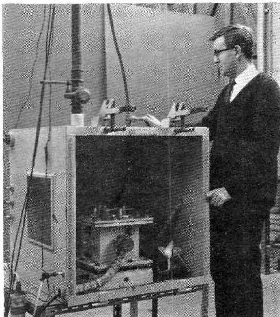
Fig. 2.—The enclosure with the  $\frac{1}{8}$  ft<sup>3</sup> explosion vessel in position
