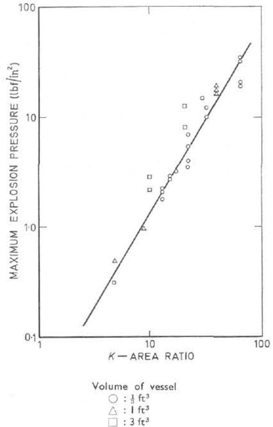
Fig. 6.—Relationship between vent area and the maximum explosion pressure for vessels with vents covered by arresters
