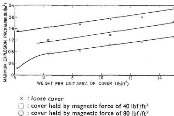
Fig. 10.—Relationship between maximum explosion pressure and the weight of the vent cover or the weight of vent cover plus magnetic force for  $\frac{1}{3}$  ft<sup>3</sup> explosion vessel with a single vent of 4.3 in. diam
