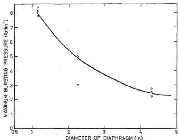
Fig. 9.—Relationship between the diameter of the diaphragm and the bursting pressure for  $\frac{1}{3}$  ft<sup>3</sup> explosion vessel without arresters
