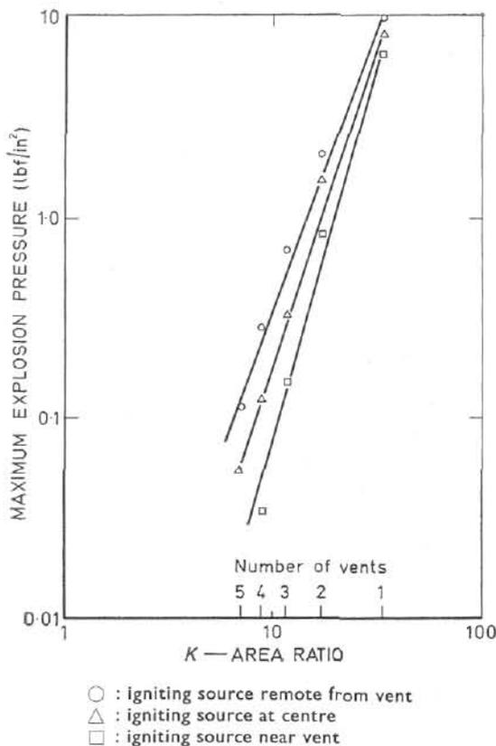
Fig. 5.—Relationship between vent area and the maximum explosion pressure for 1 ft<sup>3</sup> vessel
