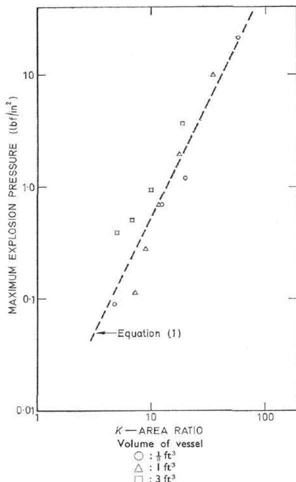
Fig. 4.—Relationship between vent area and the maximum explosion pressure
