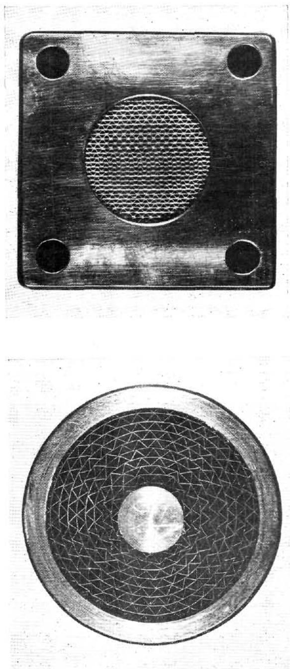
Fig. 3.—Two types of arrester. UPPER: nickel arrester. LOWER: cupro-nickel arrester.
