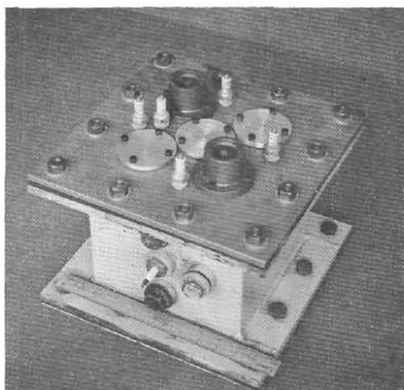
Fig. 1.— $\frac{1}{2}$  ft<sup>3</sup> explosion vessel with covers attached
