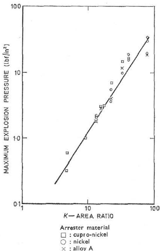
Fig. 7.—Relationship between vent area and the maximum explosion pressure for  $\frac{1}{3}$  and  $1 \text{ ft}^3$  vessels with vents covered by arresters made of different materials
