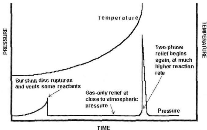
The extreme case of the situation shown in Figure 1 is the DIERS gassy reaction assumptions. These are essentially that gas-only relief (no mass loss of reactants) occurs for the whole of the runaway except that two-phase relief begins just as the reaction rate reaches its peak. Most real situations will not be as bad as DIERS assumptions. Either some two-phase relief will occur prior to the peak reaction rate being attained, or gas only relief will occur for the entire duration of the runaway.
