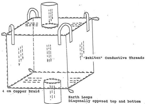
Figure 1 : Antistatic FIBC
