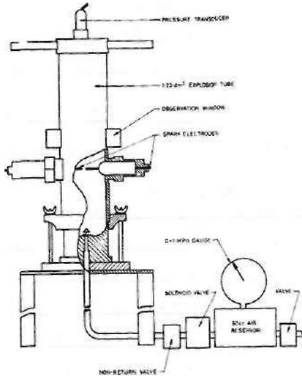
Figure 1 Hartmann vertical tube apparatus.
