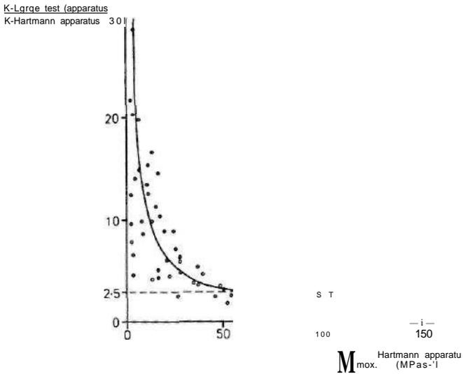
Figure 2 Comparison of Hartmann and large volume dust explosibility data - reference 1.
