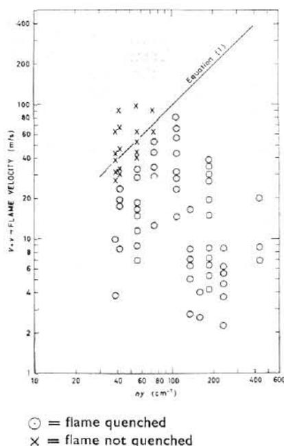
Fig. 7.—The quenching of flames ignited near the open end of the ducting
