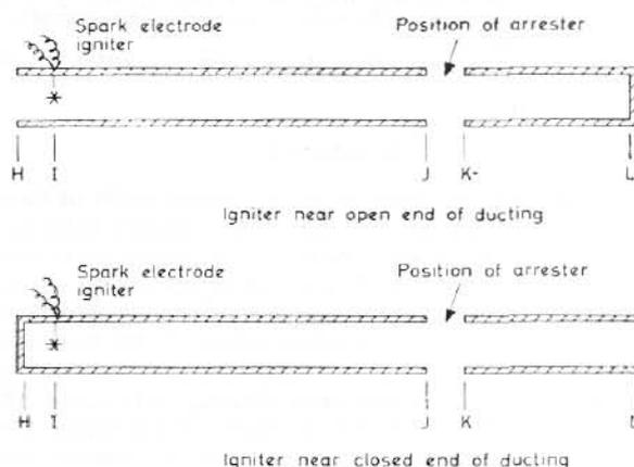
Fig. 3.—Positions of the igniter in experiments with straight ducting (not to scale)
