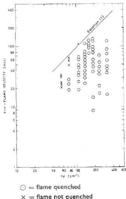
Fig. 8.—The quenching of flames ignited near the closed end of the straight ducting, without obstructions
