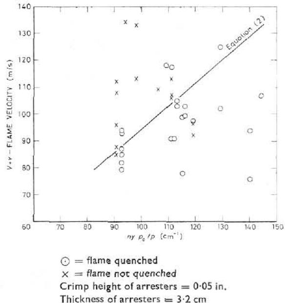
Fig. 9.—The quenching of flames ignited near the closed end of ducting with a bend or obstruction
