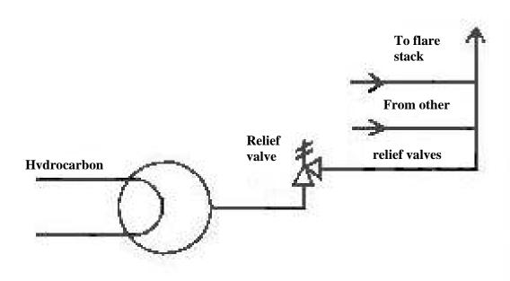
When another relief valve lifted hydrocarbon vapour came back along the discharge pipe and out of the drain hole.
