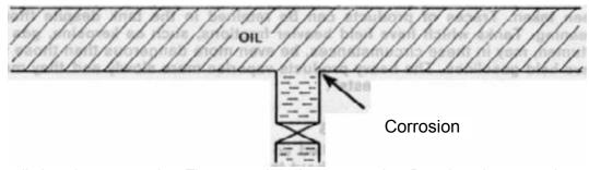
The oil alone is not corrosive. The water alone is not corrosive. But when they meet the water may react with impurities in the oil to produce corrosive products. For example, if water is added to an oil line through a branch, rapid corrosion can occur at the welds.
