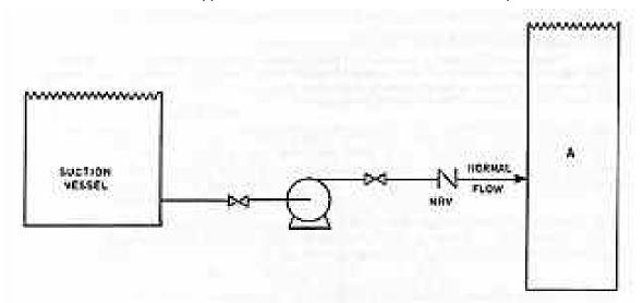
The pump tripped out. The non-return valve failed to work and the pump was driven backwards by the pressure and head of liquid in vessel A. The impellor disintegrated and the motor was damaged.
