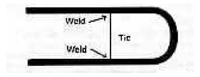
When the pipeline was complete they forgot to remove the tie and the laggers covered up the ends of it.
