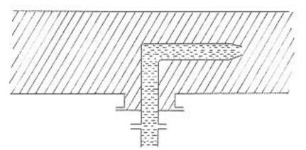
The dimensions of the branch and quill are chosen so that the injection pipe can be removed for inspection.
