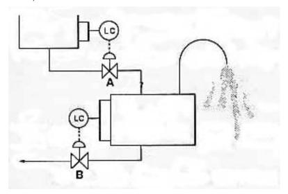
The plant was an old one. Nowadays we would fit a high level alarm on the tank. In addition, the operability study (see Newsletter 27, Item 8) would show up the fact that valve A can pass more than valve B, so its size could be reduced.
