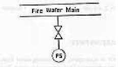
When the pressure in the main falls it is detected by the pressure switch and a pump is automatically brought into service. This happens about ten times per year. In addition, the system is tested about ten times per year to make sure it is working. Calculations show that we can expect the system to fail to work when needed once in 3.2 years.
