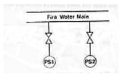
The impulse line has been duplicated as well as the pressure switch and the system will fail to work when needed once every 77 years.
