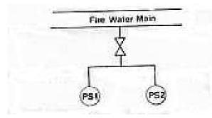
Surprisingly, this system is not much more reliable. It will fail to work on demand once every four years. This is because the most likely fault in the system is the choking of the impulse line and duplication of the pressure switch has not affected this.
