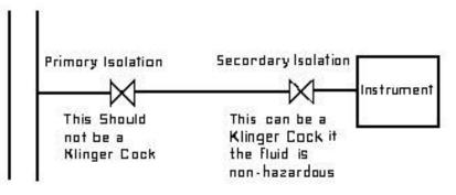
On new plants the first or primary isolation has to be made to the same specification as the main pipeline and cannot be a Klinger cock.
