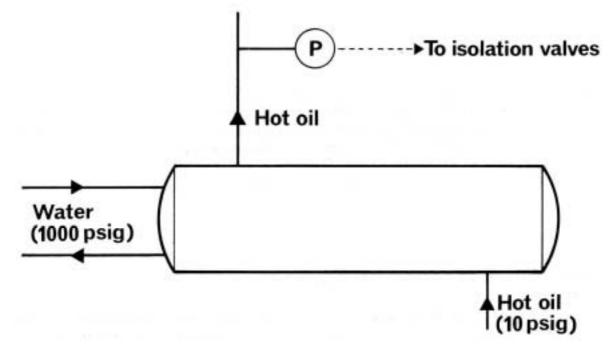
If a tube leaks water will leak into the oil and will very quickly turned into steam, causing a rapid rise of pressure
