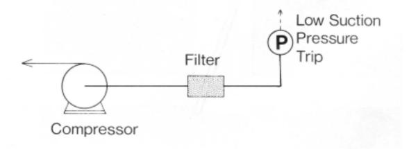
The fitter was located between the compressor and the low suction pressure trip. The fitter became choked and air was sucked into the compressor, either through leaking glands or leaking joints.
