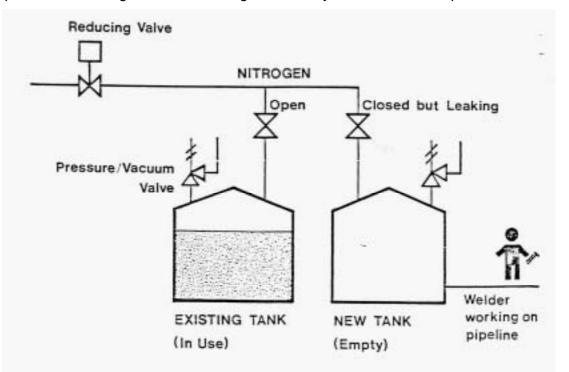
Now another similar incident has occurred. A grinder was being used near the open end of a new pipeline. Unknown to the plant people the contractors had connected up the other end of the pipeline to a live line. The connecting valve leaked, gas came out of the open end and exploded with a loud bang.
