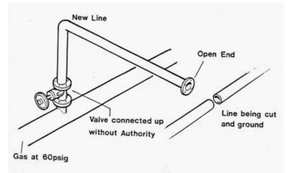
If a portable gas detector alarm (a 'Dalek') had been used it would probably have detected the leak.
