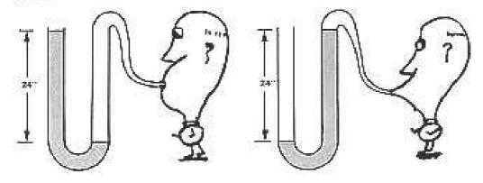
That means by just using your lungs you could over- or under-pressure a storage tank.
