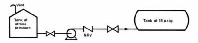
This is a good example of an accident waiting to happen. Sooner or later the non-return valve will fail and a spillage is then inevitable.
