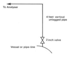
The vapour condenses in the unlagged pipe and runs back into the vessel. The system is cheap and simple and has a much shorter response time than the more elaborate systems.
