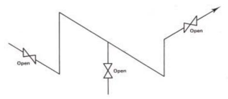
If the two block valves and the drain valve had been near each other the operator would have seen that the drain valve was open when he opened the main valves.
