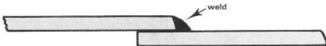
It is believed that some petrol entered the space between the plates and became trapped by rust and scale. The heat from the welding vaporised the petrol and the rise in pressure blew it out of the molten weld. If tanks made from lap-welded plates have to be repaired then they should be filled with water. The water will keep the space between the plates cool and prevent any trapped petrol vaporising.
