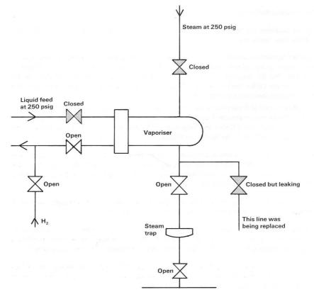
There were two leaking tubes in the vaporiser. Hydrogen entered the shell and passed through the closed steam trap by-pass valve. When a joint was broken the hydrogen escaped and caught fire. The source of ignition may have been the impact of a hammer on the bolts.
