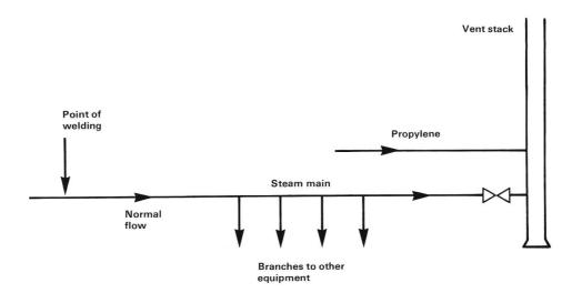
When equipment is prepared for maintenance we slip-plate or disconnect lines leading to other items of equipment. We must not overlook blowdown lines and the lines that take products to storage.
