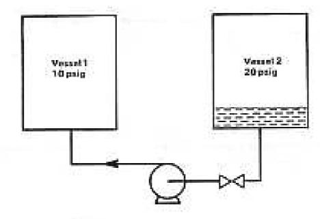
A small quantity of liquid is transferred from vessel 2 into vessel 1. The reduction in the volume of the nitrogen is small and can be neglected.
