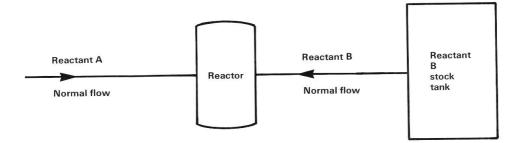
One incident was described in "Hydrocarbon Processing", March 1973, p.113. Paraffin wax and chlorine were reacted at atmospheric pressure. Some paraffin wax travelled from the reactor back up the chlorine line and reacted with liquid chlorine in a catchpot that had been installed to collect residue. The catchpot exploded with great violence — bits were found 100 feet away — and other equipment was seriously damaged.
