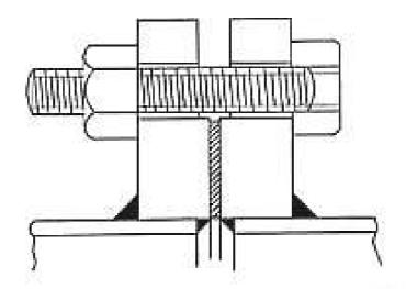
Nobody knows why this had been done. Probably one nut was tighter than the other and, in attempting to tighten this nut, the whole stud was screwed through the second nut. Whatever the reason it produced a dangerous situation as the pressure on different parts of the flange was not the same.
