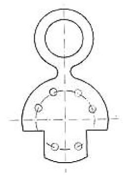
All but two of the bolts joining the relief valve to the flare header are removed; the sealing plate is then inserted and secured by special bolts with small heads that pass through the bolt holes in the relief valve flange, but not through the holes in the sealing plate. The last two bolts can then be removed and the relief valve removed. To replace the relief valve, the procedure is reversed. For details see Engineering Standard TDB 2411.
