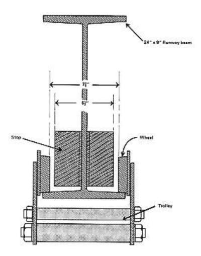
However, the biggest load that had to be lifted was 1 ton, so the runner was changed for a smaller one. It had thinner wheels which ran past the end stop and the runner fell off the end of the beam.
