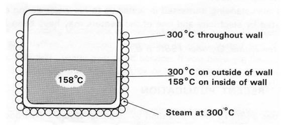
When the steam was isolated and, 15 minutes later, the stirrer switched off, the reactor walls below the liquid level fell to the same temperature as the liquid, 158°C. The reactor walls above the liquid level remained hotter. Heat passed by conduction and radiation from the walls to the top 10 cm or so of the liquid which became hot enough for a runaway reaction to start.
