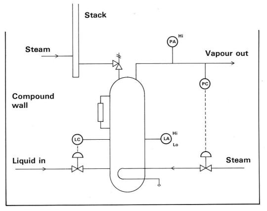
The circumstances leading up to the incident are not 100% clear but it seems that the level controller failed, so that the vaporiser filled with liquid which passed through the relief valve into the stack which then overflowed. The steam supply to the vaporiser froze but this may have occurred after the spillage due to contact with cold LPG.
