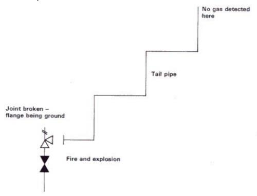
Gas in the tail pipe — 20 m long and containing a number of bends — had not dispersed and had not been detected by a test at the other end of the pipe.
