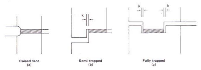
In general, when metal-jacketted gaskets are specified in the design of raised face joints as in (a), caf should not be used as a substitute. Spirally wound joints to BS 3381 incorporating an outer ring to carry the radial pressure load would be suitable.
