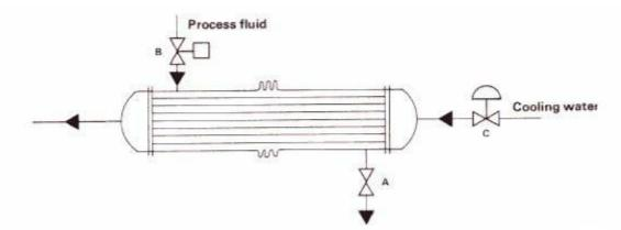
While a plant was being shut down the hot process (shell-side) flow was stopped by closing the manual isolation valve A. At the same time the cooling water flow was greatly reduced by closure of control valve C. This allowed the tubes and shell to warm up to the same temperature as the process fluid. At a later stage in the procedure, a series of trips was initiated which closed the automatic tight shut-off valve B and fully opened the cooling water control valve C.
