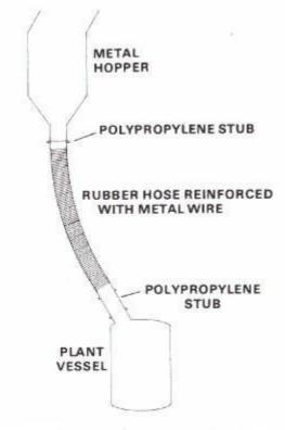
The flow of powder down the chute developed an electrostatic charge on the hose. The hose was conducting but the polypropylene end pieces prevented the charge leaking to earth. Finally, a spark occurred and ignited the dust cloud.
