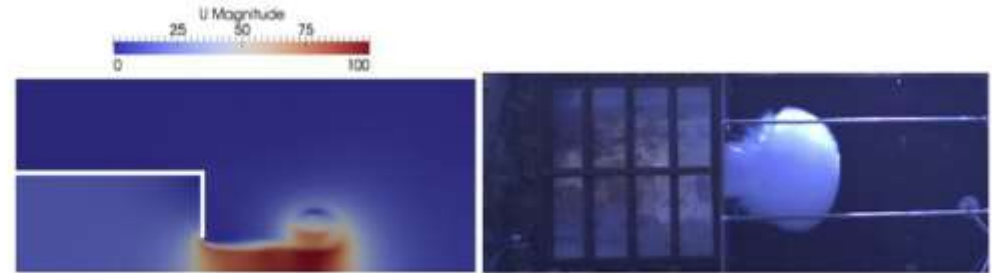
Fig. 13. Simulated flow field in front of the vent and experimental observation (test 2).
