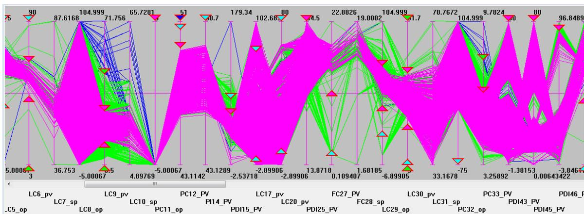
Figure 13: four sets of alarm limits with process history. Safety trip levels are shown in dark blue, hihi/lolo limits in green, hi/lo limits in red, and previous hi/lo limits in light blue. Coloration shows periods where no alarms of that class were active.
