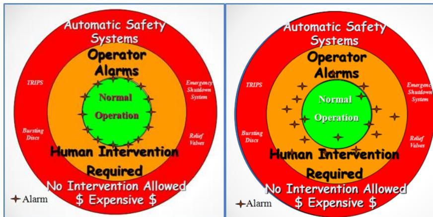
Figure 1: Schematic depiction of alarm limits. On the left, the expected configuration of alarm limits at the edge of normal operation. On the right, a more realistic picture of what is commonly seen in practice.
