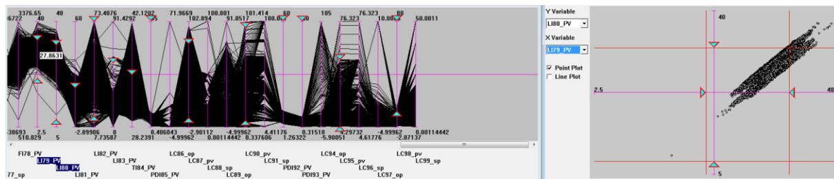
Figure 11: Redundant alarms. High alarm settings on LI79 and LI80 are at a similar level, and ring together. Low alarm settings are at two different levels.
