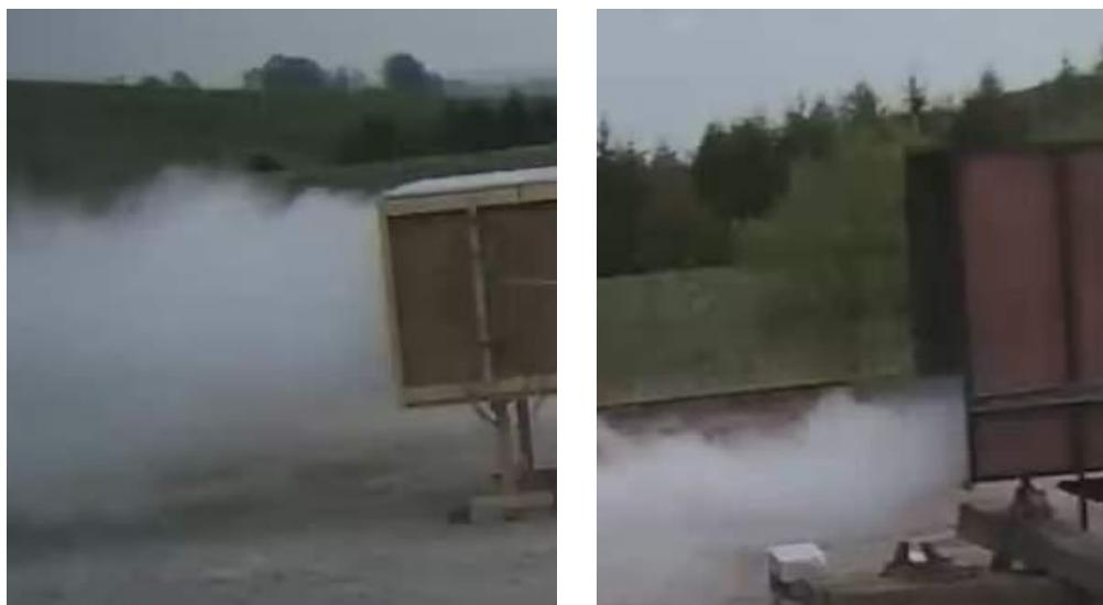
**Figure 4:** Mixed (unignited) vapour flow from the timber calibration tunnel (left) and low level unmixed gas current from the main tunnel prior to ignition in Test 2 (right)
