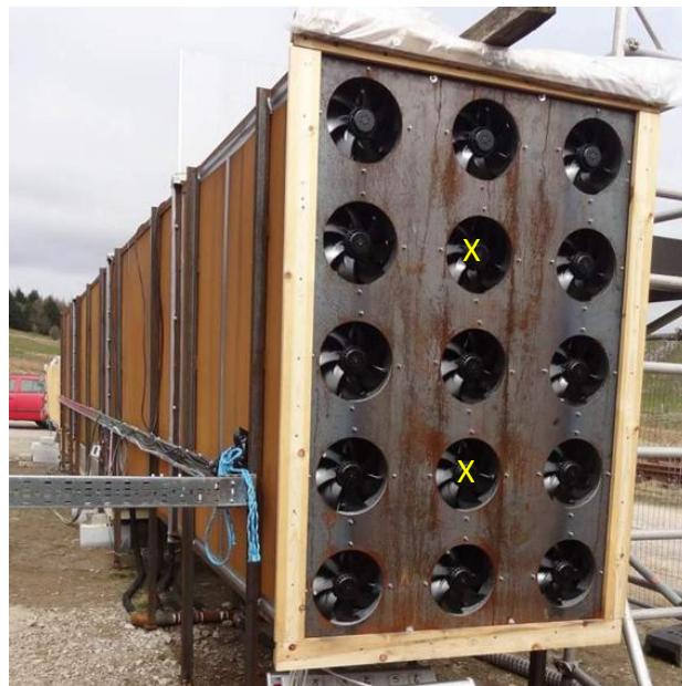
**Figure 3:** Fan array used to drive air through the tunnel
