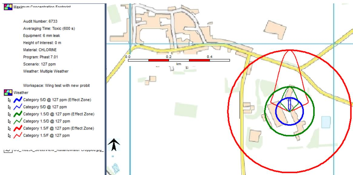
Figure 3 Maximum dispersion of cloud of 20ppm after Scenario B3
