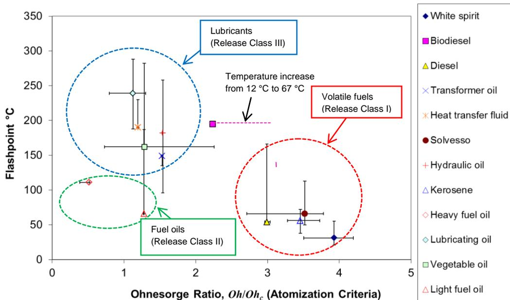
**Figure 1** Classification of stakeholder fluids by flashpoint and atomisation criteria for a 10 barg release through a 1 mm diameter orifice
