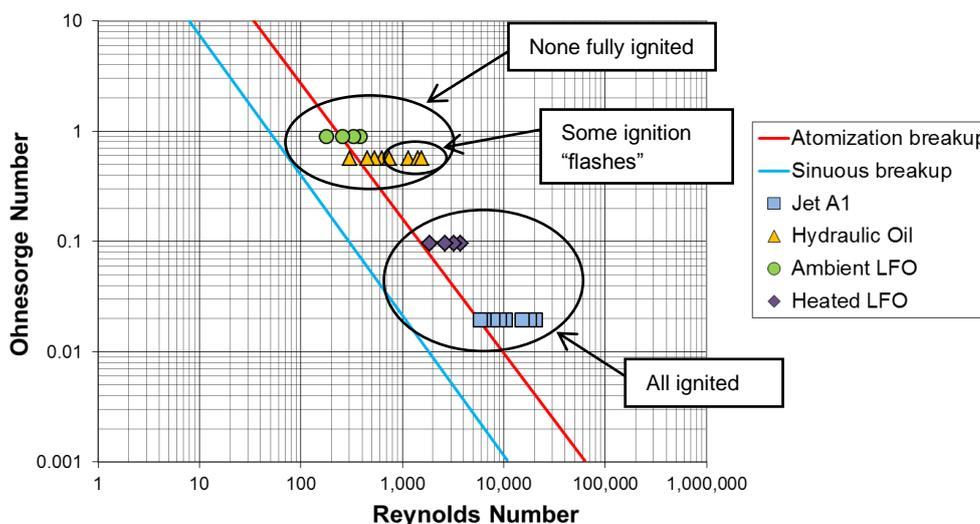
**Figure 4** Summary of conditions tested in the GTRC free spray experiments. The Reynolds number was calculated using the velocity from Bernoulli’s equation without taking into account the discharge coefficient of the orifice. The atomisation and sinuous breakup correlations were taken from Ohnesorge (1936).
