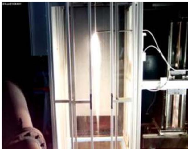
Figure 3 Photograph showing ignition of Jet A1 at a nominal release pressure of 20 barg
