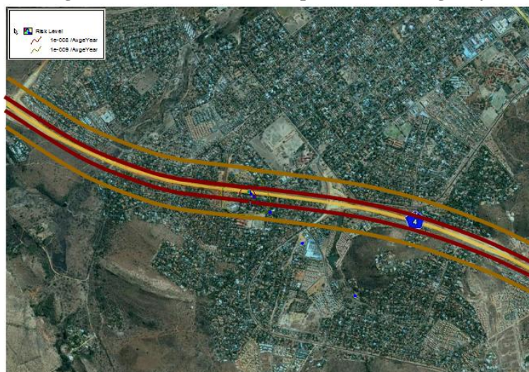
Figure 2. HF Risk Contours on part of the N4 Highway
