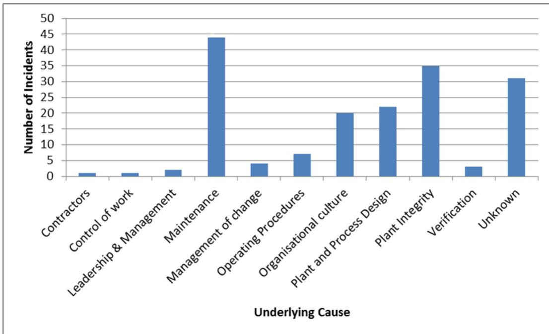
Figure 4: Underlying causes of RESDV failures.
