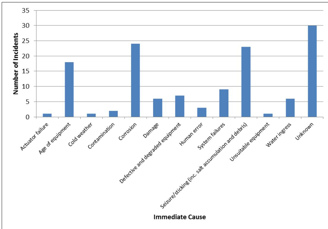
Figure 3: Immediate causes of RESDV failures.
