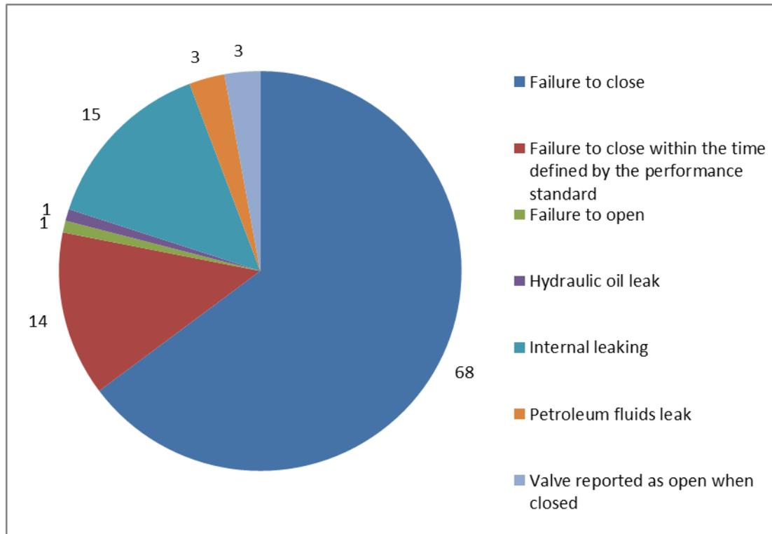
**Figure 2:** RESDV failure types.
