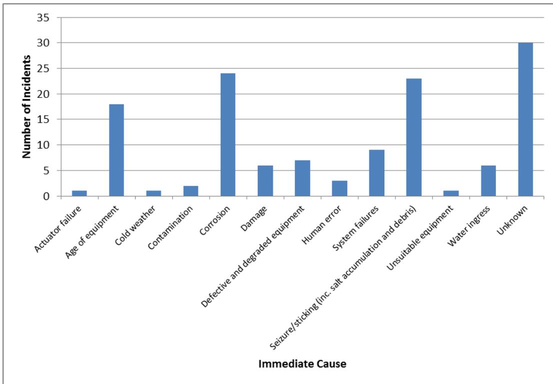
Figure 3: Immediate causes of RESDV failures.
