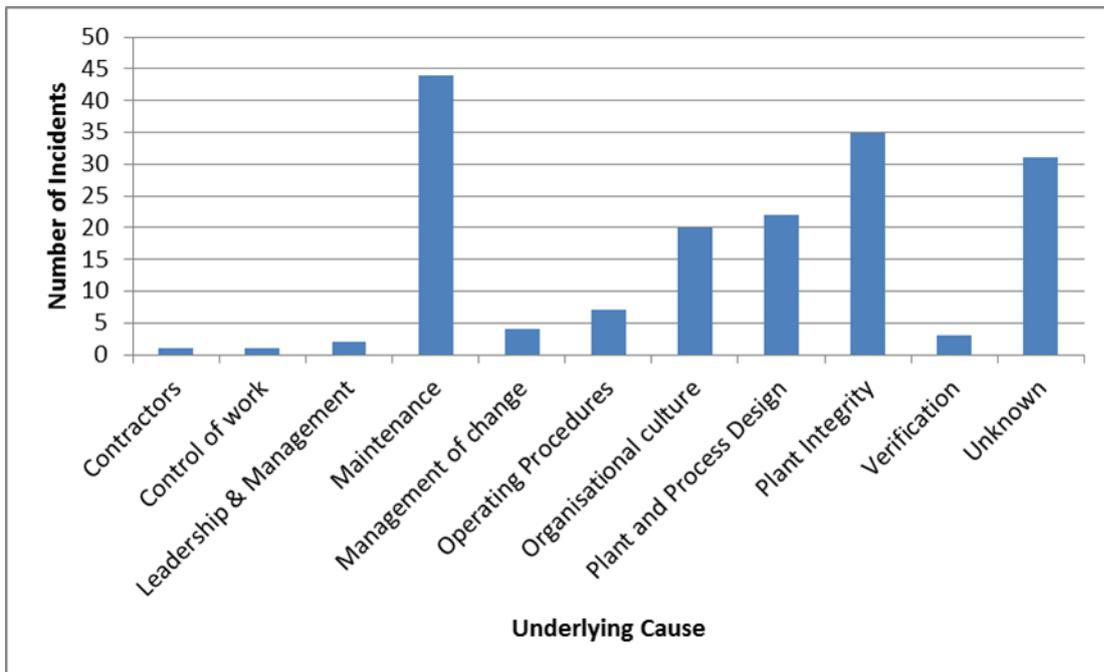
Figure 4: Underlying causes of RESDV failures.
