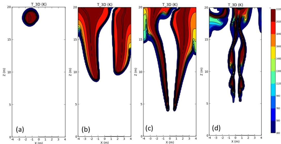
**Figure 9: Temperature field illustrates the flash fire propagating through the flammable mixture at different times after ignition. (a) 0.1 second; (b) 0.5 second; (c) 1 second; (d) 2 seconds.**
