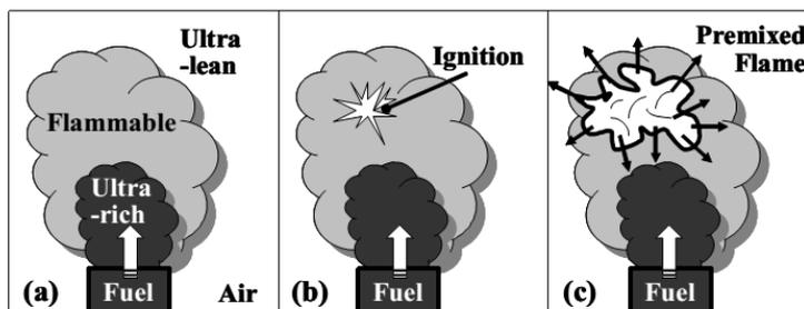
Figure 2: Problem configuration corresponding to (a) the formation of a large flammable fuel vapour cloud, followed by (b) ignition and (c) deflagration
