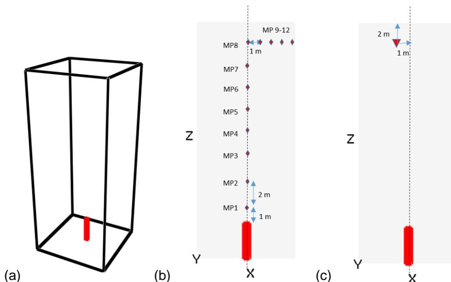
Figure 3: Numerical experiment with methane dispersed upwards: (a) 3D configuration, release from top of the red box; (b) Monitor points location in a domain central plane for dispersion verification study in Section 3, monitor point denoted by red diamonds; (c) Ignition location in a domain central plane for fire initiation, at 8s upon start of release in combustion case, location denoted by red triangle
