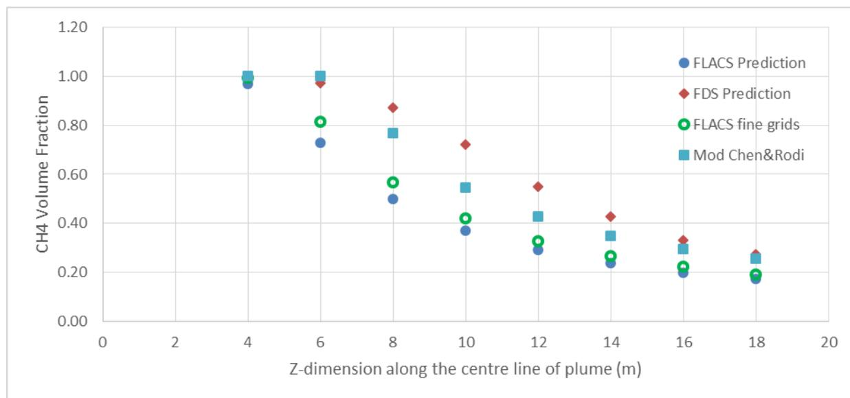
**Figure 7: Methane concentrations predicted by FDS and FLACS at centreline monitor points (MP1-MP8 as illustrated in Fig.3b), results are time-averaged between 5 and 10 seconds upon start of release. 1) Blue circle – FLACS prediction as in Fig.4; 2) Red diamond – FDS prediction as in Fig.5; 3) Green circle – FLACS prediction as in Fig.6c; 4) Blue square – modified Chen & Rodi correlation as in Eq.8 in Appendix A**
