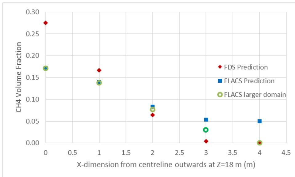
**Figure 8: Methane concentration predicted in different case at monitor points across the plume at Z=18m (MP8-MP12 as illustrated in Fig 3b). 1) Blue square – FLACS prediction as in Fig.4; 2) Red diamond – FDS prediction as in Fig.5; 3) Green circle – FLACS prediction as in Fig.6b**
