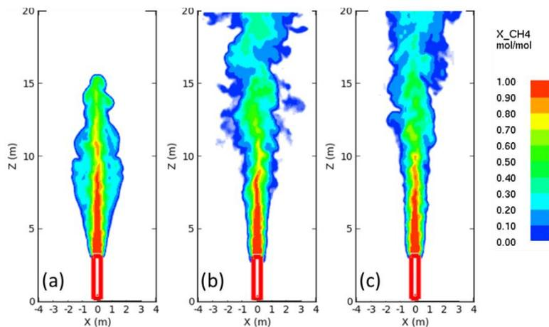
Figure 5: Methane dispersion field modelled by FDS at (a): 2 seconds; (b): 5 seconds; (c): 10 seconds, from start of release. The outer boundary of the plume denotes the LFL level, which is 5% by volume in air.
