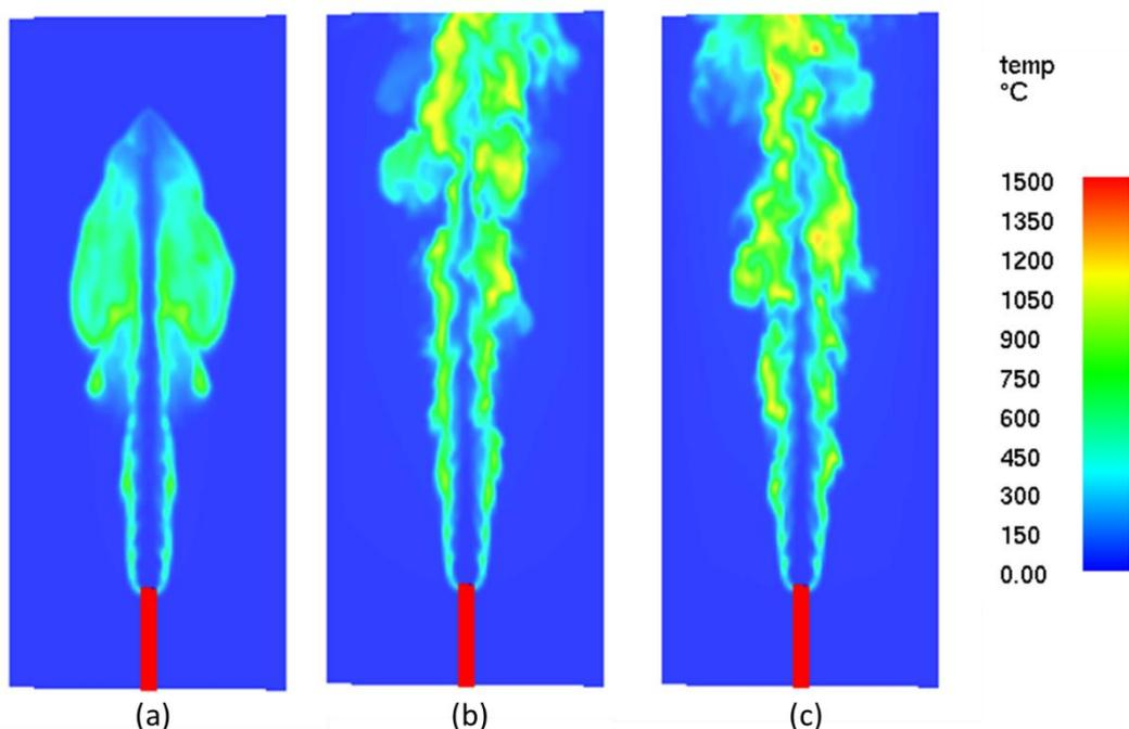
**Figure 10: Temperature field illustrates the jet fire originating from the release source upon its start on the flash-back at different time: (a) 2 seconds; (b) 5 seconds; (c) 10 seconds.**
