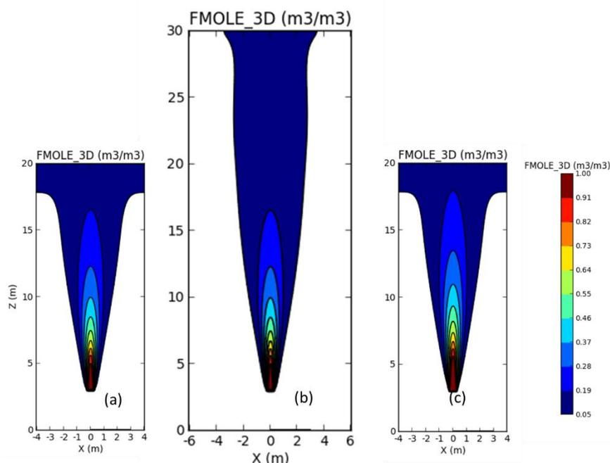
**Figure 6: Methane dispersion field modelled by FLACS at 10 seconds from start of release (a): original domain, 0.1 m grid; (b): enlarged domain, 12.2m x 12.2m x 30m, 0.1 m grid; (c): original domain, 0.05m grid. The outer boundary of the plume denotes the LFL level, which is 5% by volume in air.**
