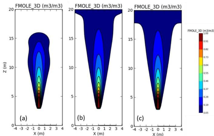
Figure 4: Methane dispersion field modelled by FLACS at (a): 2 seconds; (b): 5 seconds; (c): 10 seconds, from start of release. The outer boundary of the plume denotes the LFL level, which is 5% by volume in air.
