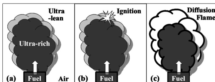
Figure 1: Problem configuration corresponding to (a) the formation of a large ultra-rich fuel vapor cloud, followed by (b) ignition and (c) diffusion burning
