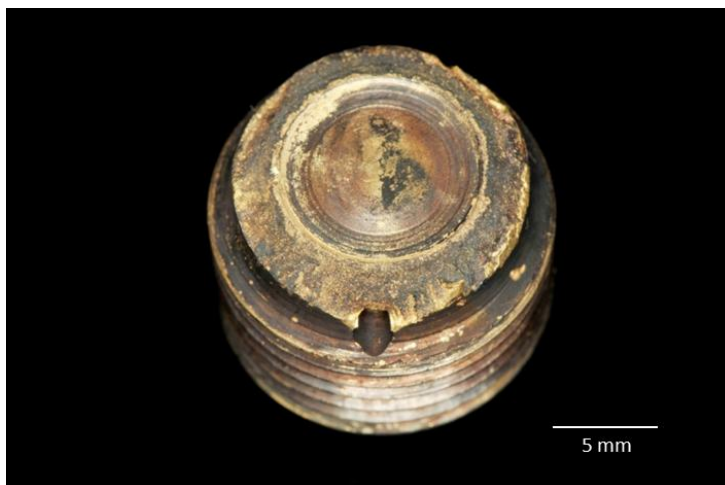
Figure 5. Inner spindle of incident valve
