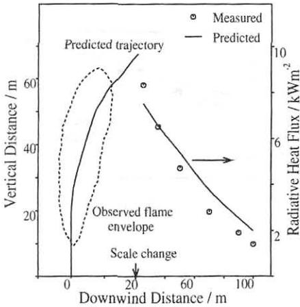
Figure 6. Flame trajectory and radiative fluxes received external to a sonic fire
