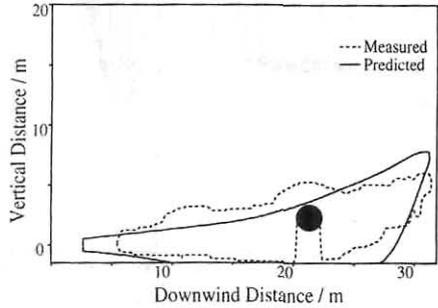
Figure 7. Flame envelopes for a sonic fire impacting a cylindrical vessel
