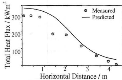
Figure 9. Total fluxes received along the stagnation line of the impacted vessel
