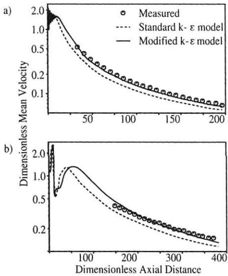
Figure 2. Decay of mean velocity in underexpanded jets with pressure ratios a) 3.1 and b) 36.9
