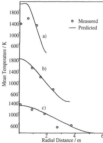
Figure 5. Radial mean temperatures in a sonic fire at a) 7.6, b) 13.1 and c) 20.4 m downstream
