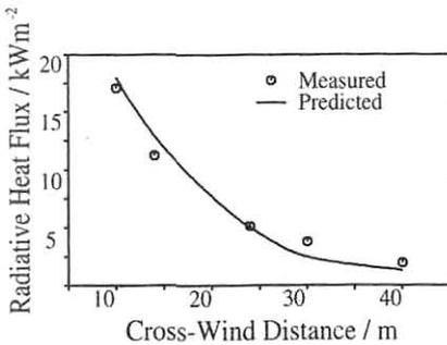
Figure 8. Radiative fluxes received external to a sonic fire
