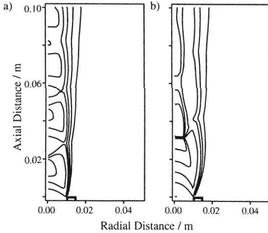
Figure 1. Predicted Mach number fields in a) moderately and b) highly underexpanded jets
