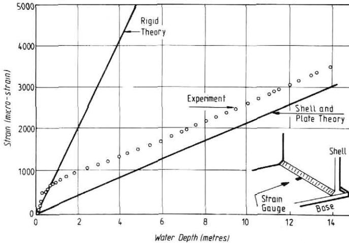
Figure 2 : Strain at the Shell to Base Junction - Water Fill
