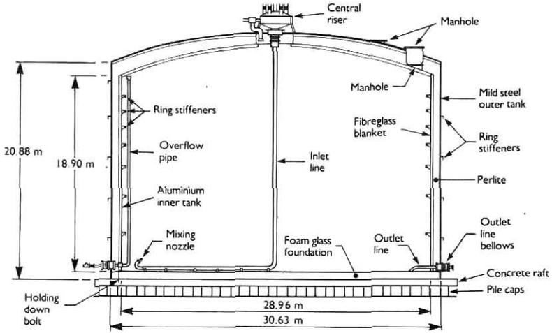
Figure 1 : Section Through Tank
