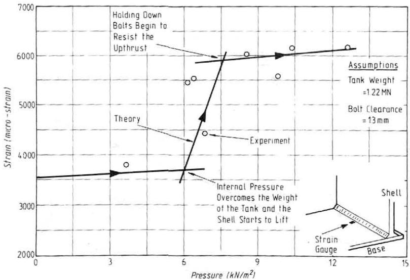
Figure 4 : Strain at the Shell to Base Junction - Internal Pressure
