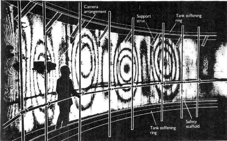
Figure 5 : Contours on the Tank Wall
