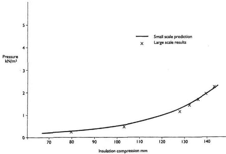
Figure 8 : Insulation Compression Characteristics
