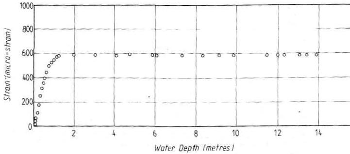
Figure 3 : Strain on Crown of Floor Bulge
