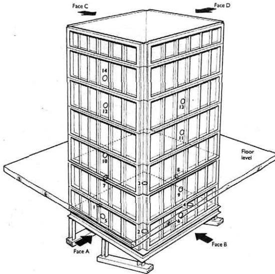
Figure 7 : Perlite Rig Showing Pressure Cell Locations
