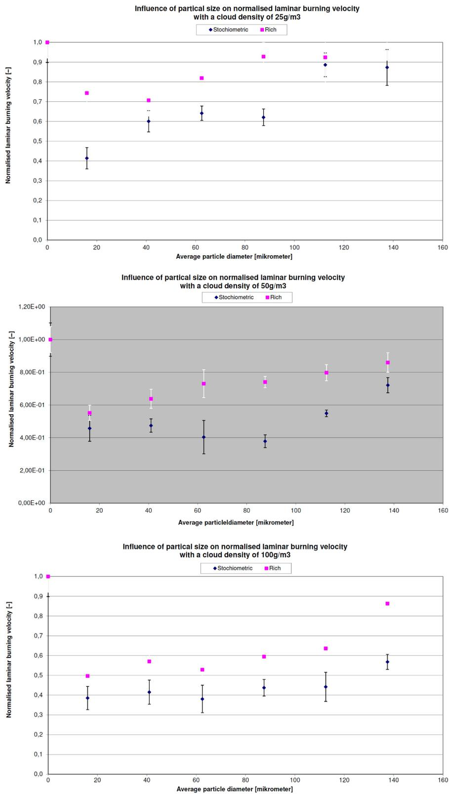
**Figure 10.** Influence of particle diameter and particle concentration on the inhibition effectiveness of potassium carbonate in propane/air-mixtures
