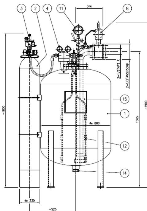
**Figure 22.** Modified mobile powder extinguishing system for use in dispersion experiments
