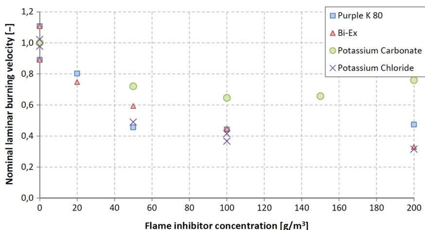
**Figure 15.** Nominal laminar burning velocities for tests with Bi-Ex, Purple K 80, KCl and K<sub>2</sub>CO<sub>3</sub> in a rich propane/air-mixture
