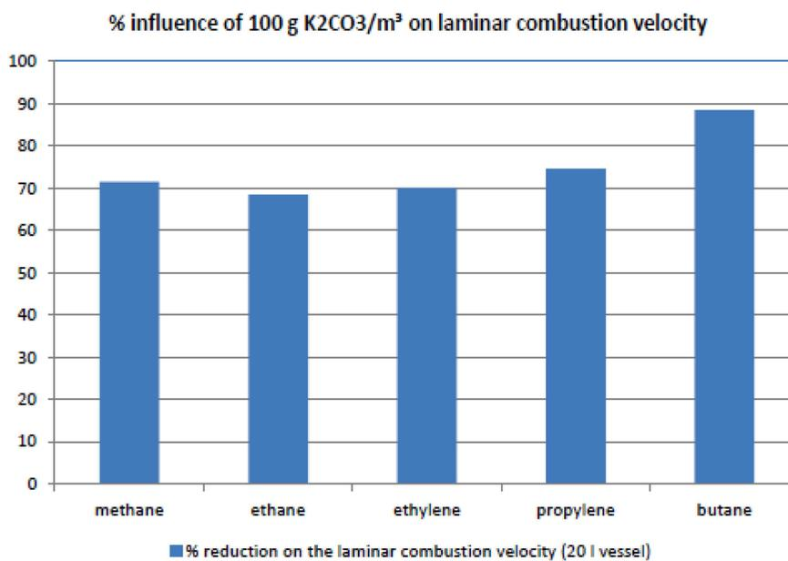
Figure 4. Influence of fuel type on inhibitor efficiency
