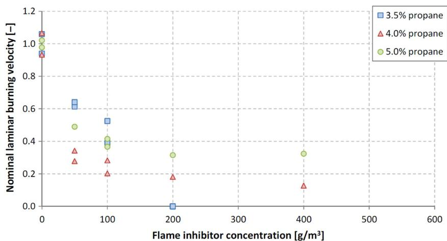
Figure 6. Nominal laminar burning velocities for tests with KCl in lean, stoichiometric and rich propane/air-mixtures
