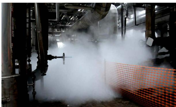
**Figure 24.** Large scale dispersion test of solid inhibitor particle cloud
