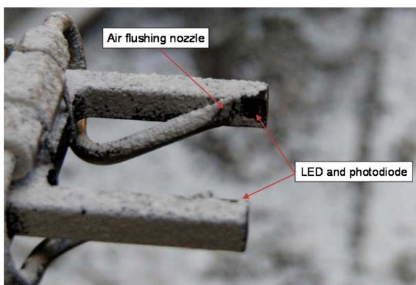
**Figure 26.** Fouling of the optics of the concentration measurement probes with inhibitor powder
