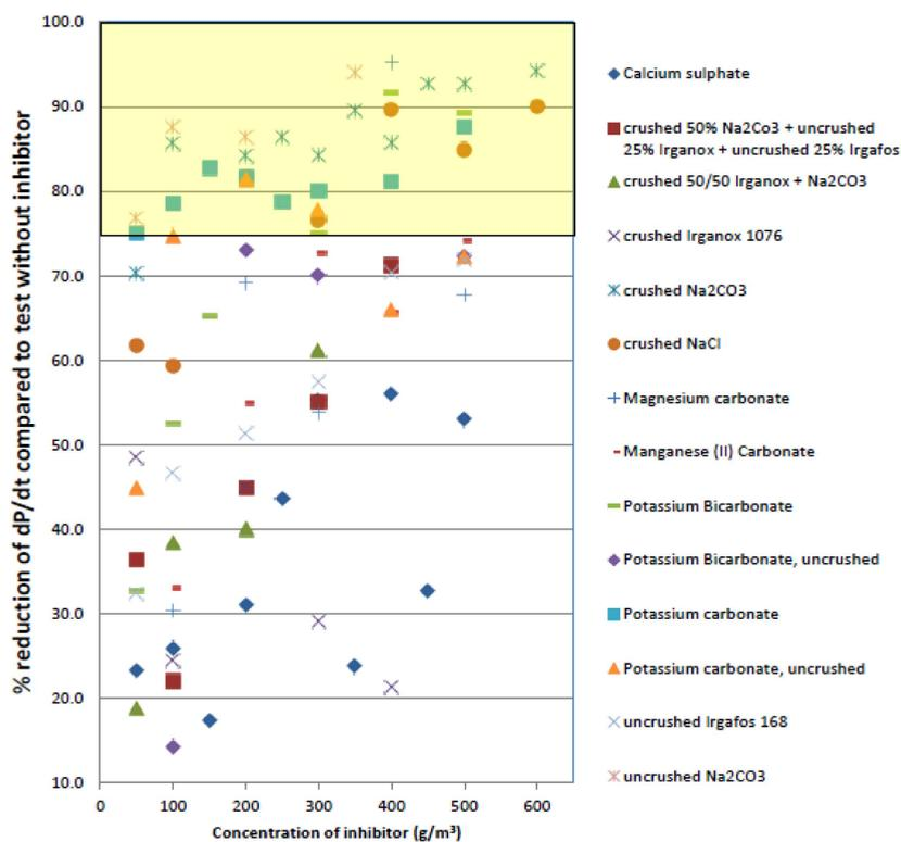
Figure 3. Pressure rise reduction for different inhibitors (propane/air-mixtures)
