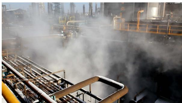
**Figure 25.** Large scale dispersion test of solid inhibitor particle cloud
