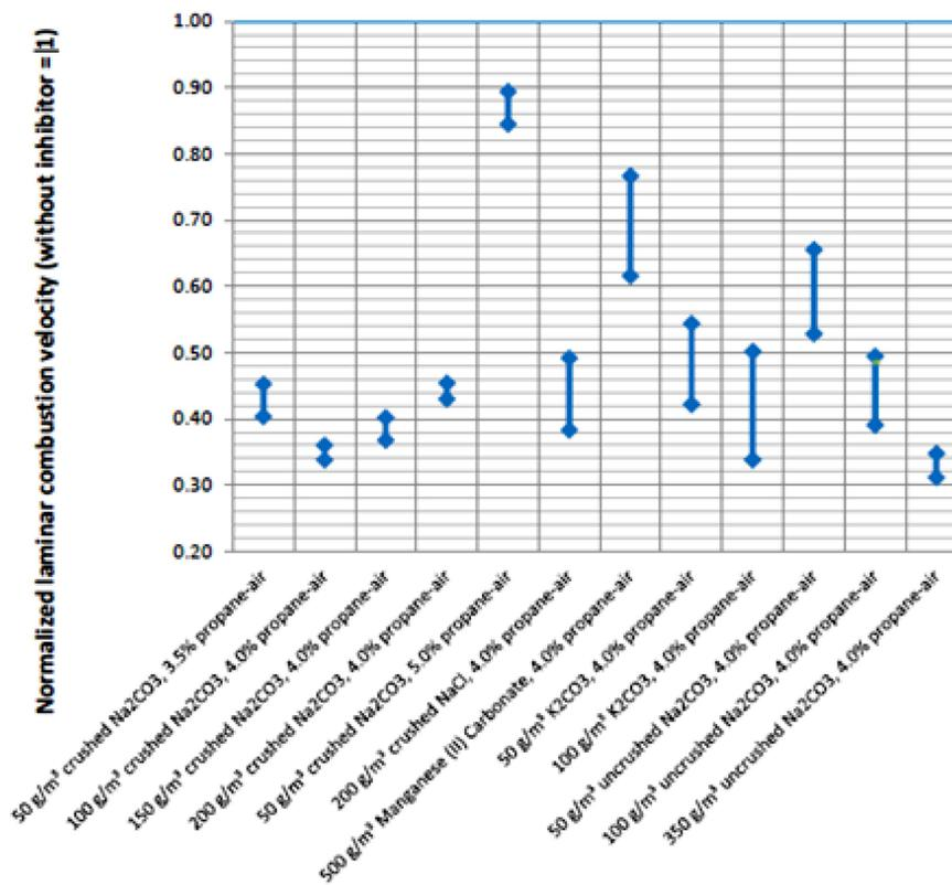
Figure 2. Influence of inhibitors on normalized laminar combustion velocity (propane/air mixtures)
