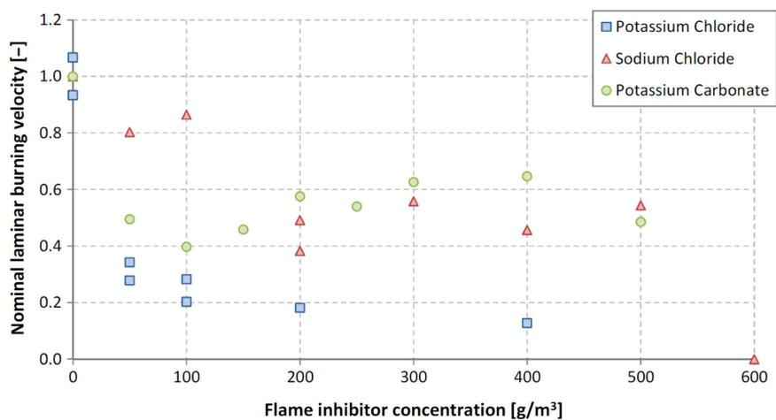
Figure 8. Nominal laminar burning velocities for tests with KCl NaCl and K<sub>2</sub>CO<sub>3</sub> in a stoichiometric propane/air-mixture
