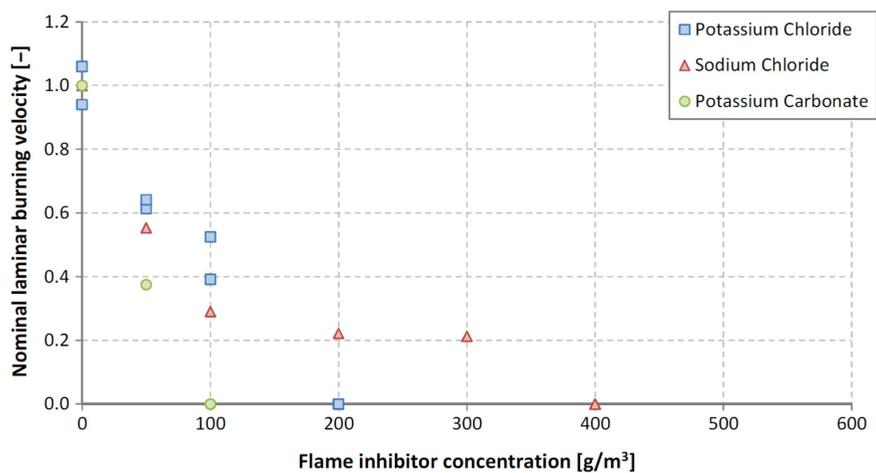
Figure 7. Nominal laminar burning velocities for tests with KCl NaCl and K<sub>2</sub>CO<sub>3</sub> in a lean propane/air-mixture
