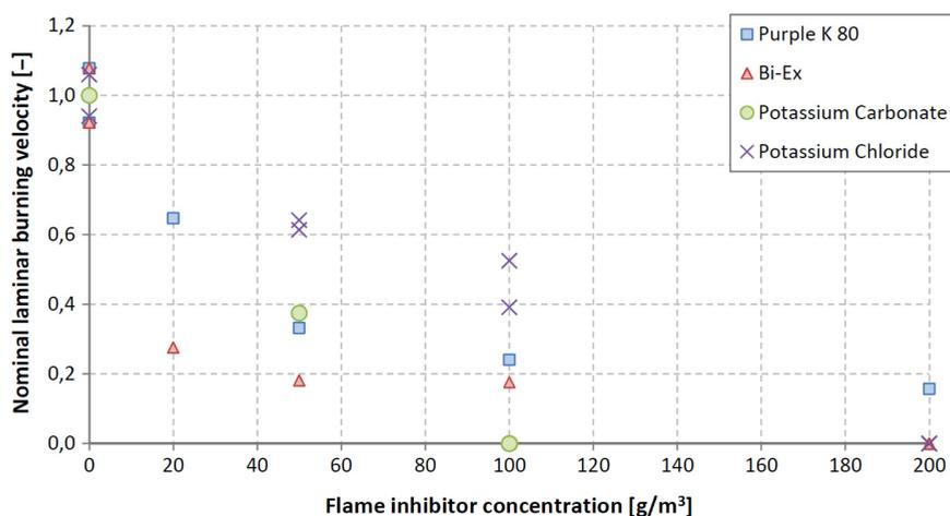
Figure 13. Nominal laminar burning velocities for tests with Bi-Ex, Purple K 80, KCl and K<sub>2</sub>CO<sub>3</sub> in a lean propane/air-mixture
