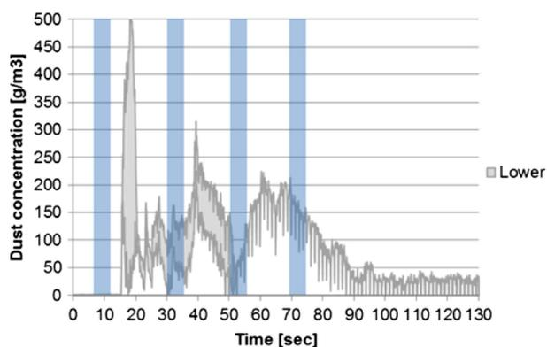
**Figure 27.** Inhibitor concentration profile measured in large scale dispersion test
