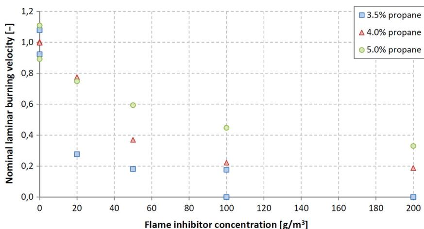
**Figure 11.** Nominal laminar burning velocities for tests with Bi-Ex in lean, stoichiometric and rich propane/air-mixtures
