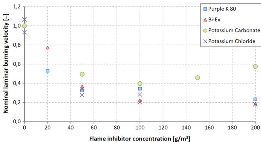
Figure 14. Nominal laminar burning velocities for tests with Bi-Ex, Purple K 80, KCl and K<sub>2</sub>CO<sub>3</sub> in a stoichiometric propane/air-mixture
