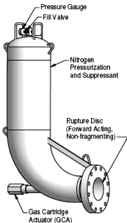
**Figure 16.** Example of explosion suppression system
