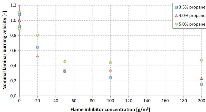
Figure 12. Nominal laminar burning velocities for tests with Purple K 80 in lean, stoichiometric and rich propane/air-mixtures
