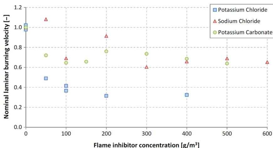
Figure 9. Nominal laminar burning velocities for tests with KCl NaCl and  $K_2CO_3$  in a rich propane/air-mixture
