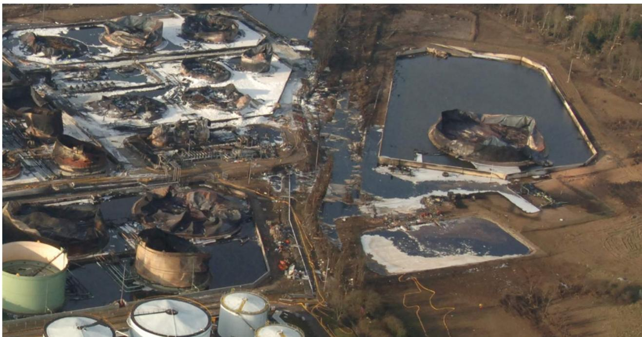
Figure 4 – Photograph taken at 12:52pm 15/12/2005 (102 hours after the explosion) (Copyright Chiltern Air Support). The photograph shows rising water levels - due to continued water use and leakage from bunds
