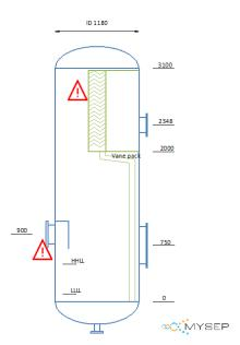
Two and three phase separators are key process equipment in Upstream, Midstream and Downstream Oil & Gas.
